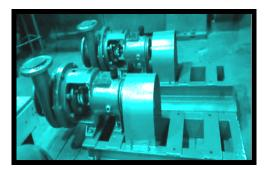
m3/hr. Total Head up to 70 meters. Temperatures up to 200 -250 Deg C in a variety of corrosion resistant metals & alloys aptly selected for your specific applications.
